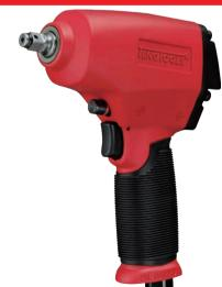
Bolt capacity - M13 Free speed - 9000rpm Forward torque (3 steps) Nm - 115 / 285 / 465 (85 / 210 / 342ft/lb) Max. reverse torque - 490Nm (361ft/lb) Min. hose size - 3/8" Air inlet - 1/4"
